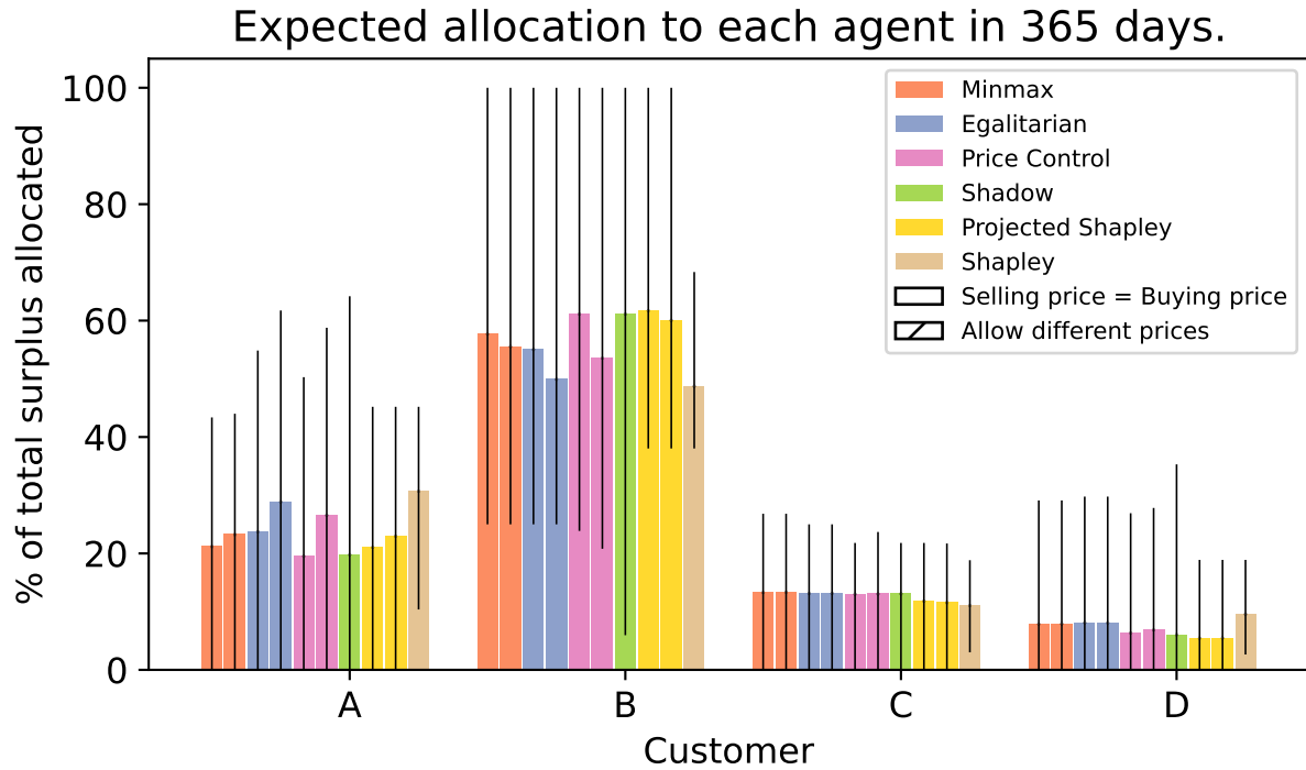
Figure 3.C.2: Proportion of savings allocated to each participant for the four mechanisms considered, case with n = 4 participants. Error bars show the range of allocations obtained during the 365 days. Main bars show the average across the year. Projected Shapley is the uniform price allocation in the core that is closest to the Shapley value in \ell_1 norm.
