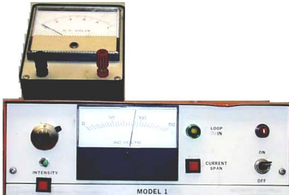
Figure 20. HV Control Interface Box, Front Panel
