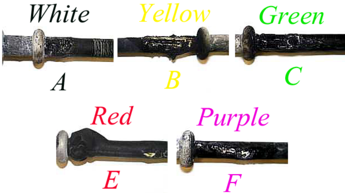
Figure 29. Series 4: damaged cable samples
